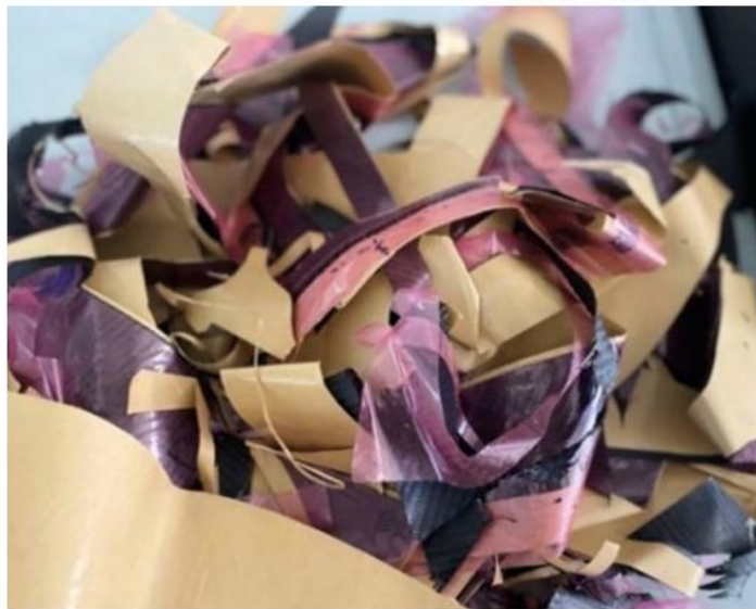
Prepreg scraps obtained from ply cutting operations.
